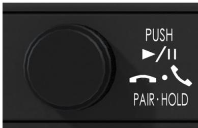
Figure 10: Front Panel Volume Knob
