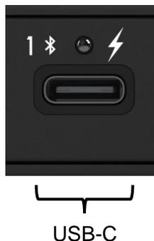
Figure 14: Front Panel USB Type C Port
