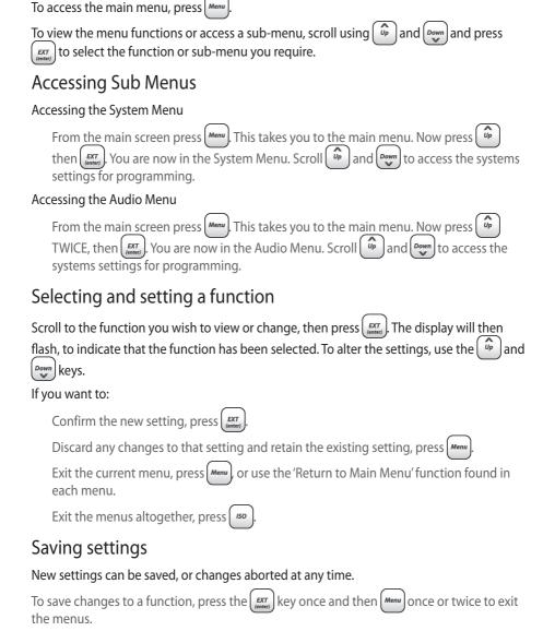
Set up the Flightcell® Pro to best suit your needs. Then from the System Menu, navigate using and pown, select 'Save user settings' and press EXT. The LCD will display
