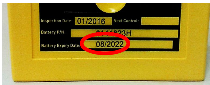
Battery expiry date on the ELT.
