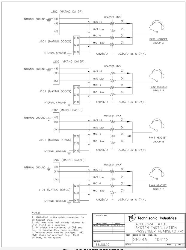
Figure 2-7 PASSENGER WIRING
