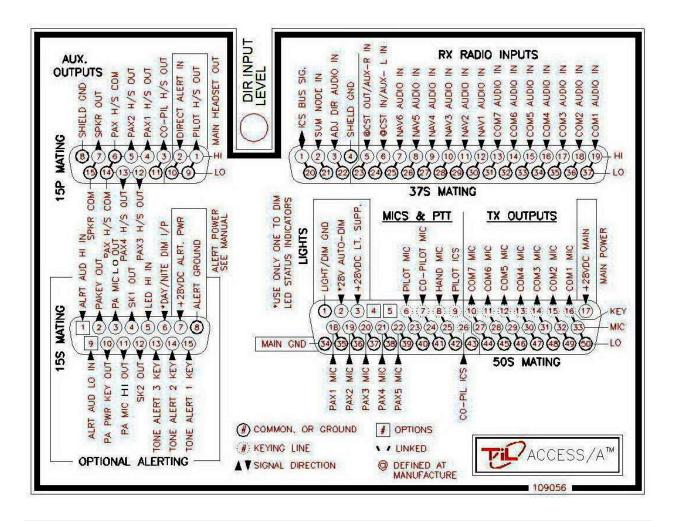
Figure 2-13 Full A711L Connector Map (view from mating connector wiring side)
