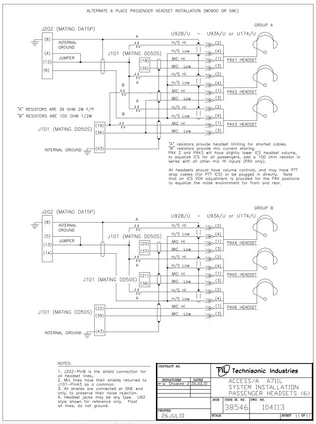
Figure 2-12 SPECIAL 6-PLACE PASSENGER WIRING
