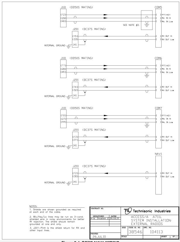
Figure 2-4 COM5-NAV1 WIRING
