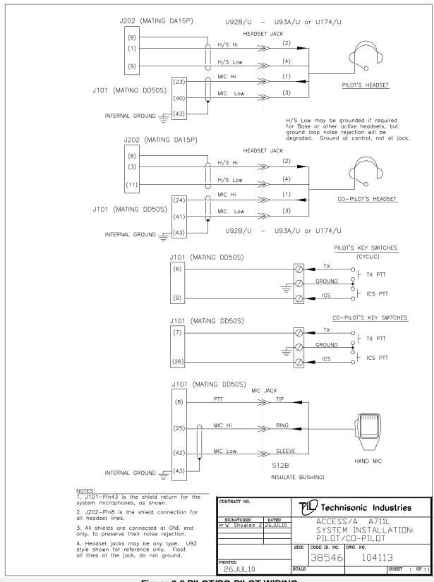
Figure 2-2 PILOT/CO-PILOT WIRING
