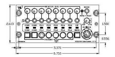
FIGURE 1-2 A711L ACCESS/A AUDIO CONTROLLER - GENERAL VIEW
