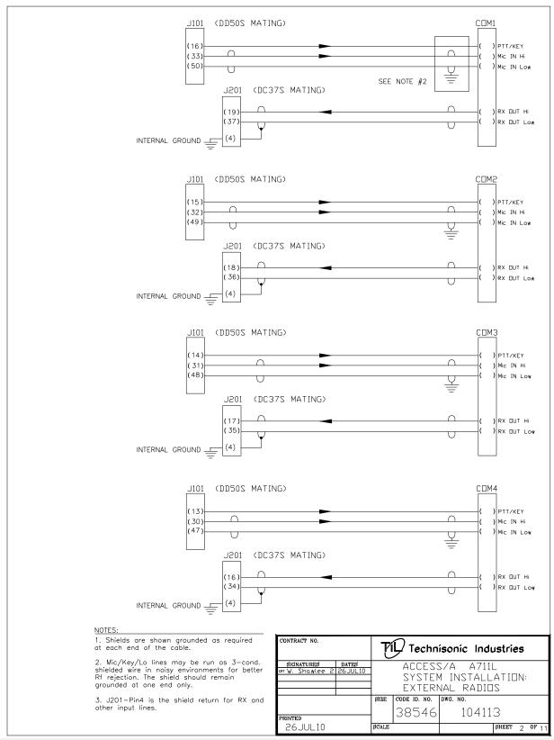
Figure 2-3 COM1-COM4 WIRING
