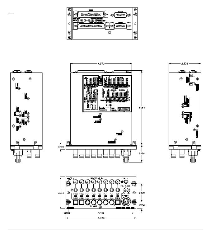
FIGURE 2-1 Outline Drawing for Model A711L ACCESS/A Audio Controller
