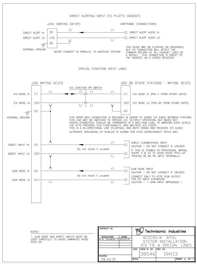
Figure 2-10 DIRECT INPUT/SPECIAL FUNCTION WIRING
