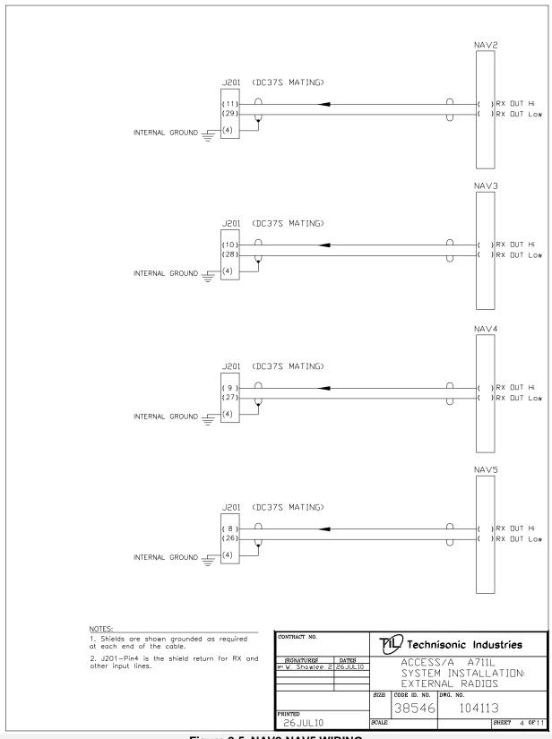
Figure 2-5 NAV2-NAV5 WIRING
