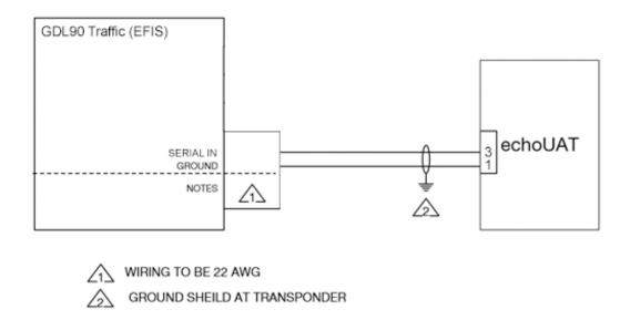
Note that in this configuration the EFIS cannot be set for control of the echoUAT Settings for Traffic on COM1 are as follows:
