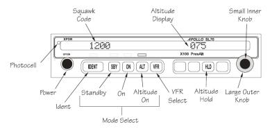
The Apollo SL70 outputs Altitude, Mode, Squawk and Mode C code over RS232. The configured baud rate needs to be determined and programmed into the echo app.
