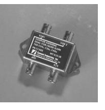
Dual VOR coupler/single glide slope diplexer allows the operation of two VOR receivers and one glide slope receiver from one VOR/glide slope antenna. Compact design makes installation easy. Also available with TNC connectors. **P/N CI 505**
