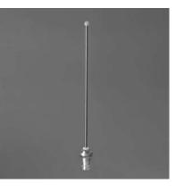
Stub antenna designed to withstand the environment associated with the underside of an aircraft. Antenna radiator is mechanically captivated and sealed against leakage. All exposed metal surfaces are nickel-plated for corrosion resistance and long service. See Order Options for connector choices. P/N CI 106
