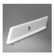
Identical to CI 118 except the mounting configuration allows for a "drop-in" replacement to the Honeywell Bendix-King™ KA26 Marker Beacon. This Comant design has been tested to the tough DO-160D environmental standards. Skydrol and rain erosion resistant. DC grounded to minimize accumulation of precipitation static. **P/N CI 118-9**
