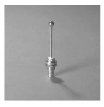
Stub-type antenna tuned for the 800-870 MHz radio telephone band. Intended for use on low-flying aircraft and helicopters. Cl 306 available with BNC connector and mounts through a single 0.600" diameter hole. Cl 306-5 available with a type N connector in which a mounting hole diameter of 0.800" is required. See Order Options for connector choices.
