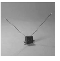
"V" Glide Slope similar to the Cl 212 except provides two output signals for dual glide slope receiver installation without the need for a glide slope coupler. Configured in a "V" for internal mounting in aircraft nose radome. **P/N Cl 212-2**
