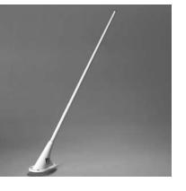
Weighs only 0.5 pounds. Features high strength fiberglass "stick" radiator and die-cast, 3-hole mounted aluminum base. Virtually identical in appearance to many Cessna communication antennas and most LORAN antennas. The CI 291 has been re-tested and upgraded to the new RTCA D0-160D environmental requirements and offers the 118 to 137 MHz frequency associated with D0-186A MOPS. **P/N CI 291**
