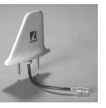
Broadband and rugged antenna designed for DME or transponder use. Antenna assembly encased in a glass reinforced polyester molded shell. Cl 105-9 comes standard with a 6" extension coax cable and BNC connector. This model offers standard two stud mounting, where the studs are extended to 1" in length. **P/N Cl 105-9**
