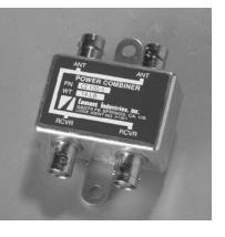
Two input—two output Power Combiner is standard equipment with Comant's CI 120-200G/S-L as supplied to Cessna. The CI 120-5 provides for two separate cable runs to the avionics installation for NAV 1 and NAV 2 receivers. P/N CI 120-5
