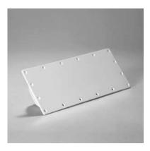
Lightweight flush mount antenna was originally designed for use on military aircraft. Provides for dual marker beacon signal outputs at the antenna, eliminating the need for a separate marker beacon splitter. Antenna is housed in an aluminum enclosure with a glass laminate cover. Internal components are potted in place for mechanical integrity. The Cl 165 is designed for flat surface mounting and is used on the Citation III<sup>TM</sup>. **P/N Cl 165**
