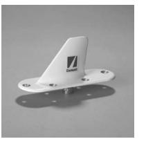
All metal, low profile antenna is designed for business jet and commercial high speed aircraft. With a popular six hole mount and connector with open path to ground, this antenna is ideally suited for those aircraft equipped with standard transponders and Mode S transponders. Tough, one piece construction provides 175 lbs. side load capability, guarding against breakage from ground equipment. Moisture failure is prevented with completely sealed construction.
