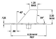
.144 DIA THRU HOLE CSK 100° x.280 DIA FAR SIDE 6 PLCS (.154 DIA HOLE REQ'D CN AIRCRAFT 6 PLCS)
