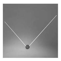
"V" Dipole VOR/Glide Slope Antenna with Fixed Elements is approved for use on helicopter aircraft. Features an integral ferrite balun and fixed element construction. Mechanically designed to withstand the severe low frequency vibration environment experienced in typical helicopter installations. APPROVED for use on helicopter aircraft. **P/N CI 259E**
