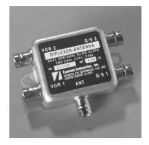
Dual VOR/dual glide slope diplexer features diplexer circuitry in a small die-stamped housing for high reliability. Provides operation between two VOR receivers and two glide slope receivers from the same VOR/glide slope antenna. **P/N CI 1125**
