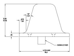
.201 DIA THRU HOLE CBORE .359 DIA FAR SIDE 4 PLCS (.203 DIA HOLE REQ'D ON AIRCRAFT 4 PLCS)
