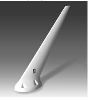
First of its kind, the CI 2680-504 combines four separate antenna functions into one. Three different connectors are on the base plate; TNC for GPS, SMA for popular satellite radio and/or weather data systems, and BNC for combined VHF/Orbcomm. The BNC VHF/Orbcomm requires the Avidyne DC50 Coupler®, allowing the VHF side to operate as Comm 2 or as Orbcomm TX/RX.
