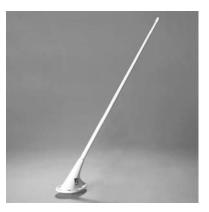
Similar to the Cl 109, the Cl 121 is smaller in diameter and lighter at only 0.5 pounds. Features a tapered glass laminate housing and die-cast aluminum base. Offers standard mounting and appearance to many Cessna communication antennas. The Cl 121 has been re-tested and upgraded to the new RTCA D0-160D environmental requirements and offers the 118 to 137 MHz frequency associated with D0-186A MOPS.
