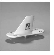
All metal, low profile antenna is designed for business jet and commercial high speed aircraft. With a popular four hole mount and connector with open path to ground, this antenna is ideally suited for those aircraft equipped with standard transponders and Mode S transponders. Tough, one piece construction provides 175 lbs. side load capability, guarding against breakage from ground equipment. Moisture failure is prevented with completely sealed construction.
