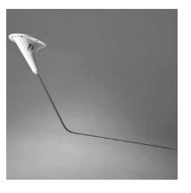
Designed specifically for mounting to the underside of an aircraft providing excellent radiation coverage for air-to-ground communications. Bent configuration makes it ideally suited for helicopters and low wing aircraft. The CI 122 has been re-tested and upgraded to the new RTCA D0-160D environmental requirements and offers the 118 to 137 MHz frequency associated with D0-186A MOPS.
