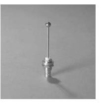
Transponder antenna with top loaded stub monopole. Antenna radiator is mechanically captivated and is machined from solid brass for impact resistance. Contact points are made from beryllium copper. Metallic parts are plated with bright nickel for corrosion protection. Mounts through a single 0.600" diameter mounting hole.
