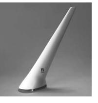
Designed for large single or twin-engine aircraft. The antenna assembly enclosed in an aerodynamically shaped, injection molded polyester glass shell with internal components foamed in place for mechanical integrity. Reduced height convenient for mounting to the underside of an aircraft. The 119 has been re-tested and upgraded to the new RTCA D0-160D environmental requirements and offers the 118 to 137 MHz frequency associated with D0-186A MOPS.
