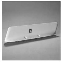
Identical to CI 118 except the mounting base includes a flange to provide for 4-hole external mounting. Approved for medium to high-performance single, turbo-prop or jet aircraft and provides simple external mounting. Skydrol and rain erosion resistant. DC grounded to minimize accumulation of precipitation static. **P/N CI 118-5**
