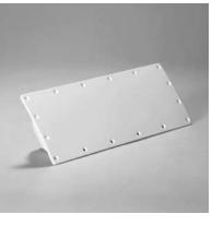
Lightweight flush mount antenna was originally designed for use on military aircraft. Provides for dual marker beacon signal outputs at the antenna, eliminating the need for a separate marker beacon splitter. Antenna is housed in an aluminum enclosure with a glass laminate cover. Internal components are potted in place for mechanical integrity. The Cl 164 is designed for curved "crown" surface mounting as is currently used on the Cessna<sup>™</sup> Citation I and II.
