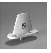
L Band/UHF blade antenna designed for high performance aircraft. Low profile, light weight antenna and is packaged in a molded body with metal mounting base to ensure stable environmental performance and resistance to vibration, rain erosion and cleaning solvents. Features vertical/omnidirectional pattern, wide band/high efficiency electrical performance and DC grounding for lightning protection. See Order Options for connector choices. **P/N CI 310 Series**
