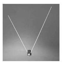
"V" Dipole VOR/Glide Slope Antenna with detachable elements was developed specifically for Commander aircraft. Mounts inside top of vertical stabilizer for improved aerodynamics. RF design is similar to the CI 157P. Integral ferrite balun provides for higher radiation efficiency. Not approved for helicopter installations. **P/N CI 182**
