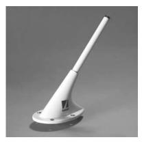
A rugged monopole antenna particularly well-suited to the harsh environments experienced on the underside of an aircraft. Features standard 4-hole mounting, die-cast metal base and radiator encased in glass laminate housing. **P/N CI 177-20**
