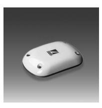
Completely redesigned 401 Series ARINC footprints GPS. This model contains an all-new, highly stable amplifier that offers great performance. Gain performance at 26.5 to 31.5 dB provides excellent Satcom rejection at 40 dB minimum. Plus, this antenna presents very low noise levels at 3.8 dB maximum.
