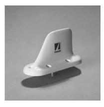
Similar to the Cl 105-20 series but offers slightly lower profile. Wide band vertically polarized/omnidirectional antenna designed for high performance aircraft over the UHF/L band of frequencies. Features 6-hole mounting, low drag, low weight, wide band/high efficiency electrical performance, DC grounding for lightning protection and Skydrol/rain erosion resistance.
