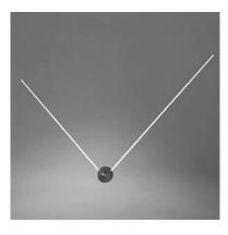
"V" Dipole VOR/Glide Slope Antenna with detachable elements was developed specifically for Beech Bonanza aircraft and encompasses reduced static capability with the use of P-Stat paint and bleeder resistors. Integral ferrite balun provides for higher radiation efficiency. Not approved for helicopter installations. **P/N CI 158C-3**
