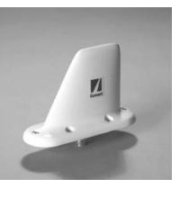
Wide band vertically polarized/omnidirectional antenna designed for high performance aircraft over the UHF/L band of frequencies from 806 to 960 MHz. Low profile blade-type construction features 6-hole mounting, low drag, low weight, wide band/high efficiency electrical performance, DC grounding for lightning protection and Skydrol/rain erosion resistance.
