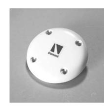
Active GPS antenna designed for airborne applications for aircraft up to 600 knots. Certified to TSO C-144, and D0-228 Minimum Operation Performance requirements. This antenna offers DC grounding and has passed rigorous Lightning Direct Effects testing as prescribed in D0-160D. Round footprint allows for drop-in replacement in many popular GPS applications. **P/N CI 408-20/Active**
