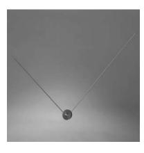
"V" Dipole VOR/Glide Slope Antenna with detachable elements mounts on top of the vertical fin stabilizer for most single engine general aviation aircraft. RF design similar to the CI 157P. Integral ferrite balun provides for higher radiation efficiency. Detachable element results in a significantly smaller shipping and storage carton than fixed element versions. Not approved for helicopter installations. **P/N CI 158C**
