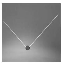
"V" Dipole VOR/Glide Slope Antenna with detachable elements is similar to the CI 158C-3 with the exception of offering 2-hole mount instead of a 4-hole mount. This V Dipole encompasses reduced static capability with the use of P-Stat paint. Integral ferrite balun provides for higher radiation efficiency. Not approved for helicopter installations.
