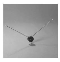
"V" glide slope designed specifically for mounting inside the nose cone of twin-engine aircraft. Provides a -3dB reduction in gain at the +30 degree points and +6.0 dB gain looking forward relative to standard glide slope antennas. Antenna radiation characteristics eliminate or significantly reduce problems associated with propeller modulation.
