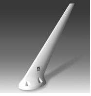
First of its kind, the CI 2680-500 combines four separate antenna functions into one. Three different connectors are on the base plate; TNC for GPS, SMA for popular satellite radio and/or weather data systems, and BNC for combined VHF/Orbcomm. The BNC VHF/Orbcomm requires the Avidyne DC50 Coupler<sup>®</sup>, allowing the VHF side to operate as Comm 2 or as Orbcomm TX/RX.
