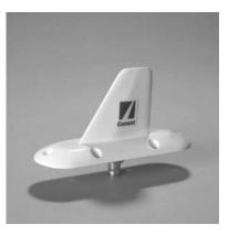
All Metal Blade DME/Transponder antenna designed and developed for Mach 2 military aircraft. Design is unique in that blade and mounting base are die-cast as one piece with no dielectric material in the airstream. Standard six-hole mounting configuration. See Order Options for available connectors. P/N CI 100 Series
