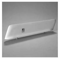
Designed specifically for high-performance aircraft applications. Features aerodynamic design in a lightweight package. Antenna is a low profile blade-type encased in a molded polyurethane shell. Skydrol and rain erosion resistant. **P/N CI 118**
