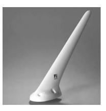
Specifically designed for medium speed single and twin-engine aircraft. Features a low drag aerodynamic blade design with an overall height of 13". The CI 238 has been re-tested and upgraded to the new RTCA D0-160D environmental requirements and offers the 118 to 137 MHz frequency associated with D0-186A MOPS. **P/N CI 238**
