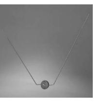
"V" Dipole VOR/Glide Slope Antenna with fixed elements designed specifically for compatibility with the Piper Aircraft mounting. Integral ferrite balun provides for higher radiation efficiency replacing cumbersome coaxial baluns previously utilized. Radiating elements are not removable. Not approved for helicopter installations.
