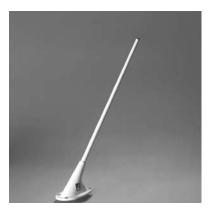
Wider band version of the Cl 177 with 2.5:1 VSWR or better over a frequency band of 138 to 174 MHz. Improved bandwidth provides greater flexibility by optimizing features of some of the newer FM transceivers. Features a molded base with popular 3-hole mounting. Radiating element is enclosed in a high strength, tapered glass laminate housing.
