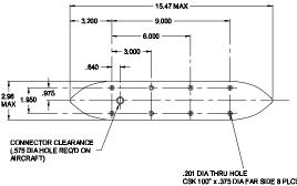
.201 DIA THRU HOLE CSK 100° x.375 DIA FAR SIDE 8 PLCS (.203 DIA HOLE REQID ON AIRCRAFT 8 PLCS)
