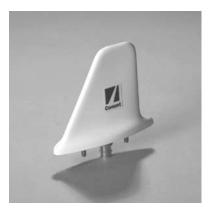
Broadband and rugged antenna designed for DME or transponder use. Antenna assembly encased in a glass reinforced polyester molded shell. Standard two stud mounting configuration. Cl 105 includes a BNC connector.
