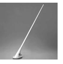
Wider band version of the Cl 177 over a frequency band of 138 to 174 MHz. Improved bandwidth provides greater flexibility by optimizing features of some of the newer FM transceivers. Features a molded base with popular 4-hole mounting. Radiating element is enclosed in a high strength, tapered glass laminate housing. **P/N Cl 177-1**
