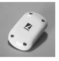
Active GPS antenna designed for airborne applications for aircraft up to 600 knots. Certified to TSO C-129a, complies to ARINC 743 specifications, and D0-208 Minimum Operation Performance requirements. All 401 Series antennas offer DC grounding and have passed rigorous Lightning Direct Effects testing as prescribed in D0-160C. Available in many standard formats as listed. Additional designs with various gain and filter configurations are available. **P/N CI 401 Series/Active**
