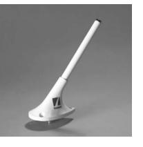
Rugged monopole antenna particularly well-suited to the harsh environments experienced on the underside of an aircraft. Features a very compact 3-hole mounted die-cast aluminum base with the radiator encased in a glass laminate housing.
