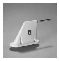
Wide band UHF antenna designed for high-performance aircraft over the full frequency range of 406-512 MHz. Low profile, blade-type antenna is encased in a low drag, low weight molded body to ensure high reliability. The CI 275 comes standard with BNC connector. Other connectors available. See order options chart. **P/N CI 275 Series**
