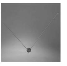
"V" Dipole VOR/Glide Slope Antenna with detachable elements mounts on top of the vertical fin stabilizer offering the four-hole mounting configuration found on many Beech aircraft. RF design similar to the CI 157P. Integral ferrite balun provides for higher radiation efficiency. Detachable element results in a significantly smaller shipping and storage carton than fixed element versions. Not approved for helicopter installations.
