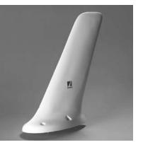
Blade-type antenna with four mounting holes for external mounting on high-performance twins and jets. Very low-drag profile and clean aerodynamical shape. Suitable for mounting on top or bottom of the aircraft fuselage. The Cl 223-1 is identical to the Cl 223 but with offset connector. The Cl 223-1 has been re-tested and upgraded to the new RTCA D0-160D environmental requirements and offers the 118 to 137 MHz frequency associated with D0-186A MOPS. **P/N Cl 223-1**
