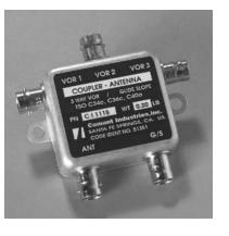
Triple VOR coupler/single glide slope diplexer allows operation between three VOR receivers and one glide slope receiver from the same VOR/glide slope antenna.
