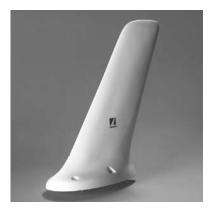
Blade-type antenna with four mounting holes for external mounting on high-performance twins and jets. Very low-drag profile and clean aerodynamical shape. Suitable for mounting on top or bottom of the aircraft fuselage. The CI 223 has beenre-tested and upgraded to the new RTCA D0-160D environmental requirements and offers the 118 to 137 MHz frequency associated with D0-186A MOPS. **P/N CI 223**
