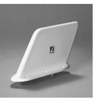
UHF blade antenna design for high performance aircraft over the full frequency range of 400-960 MHz. Low profile, low drag, light weight antenna is packaged in a molded body and metal mounting base to ensure stable performance in tough environmental conditions. Features vertically polarized/omnidirectional pattern, extremely wide band/high efficient electrical performance. DC grounding for lightning protection, 6-hole mounting.
