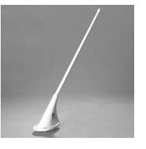
The CI 177-4 is specifically designed for use with Weather/Data or WX systems, bringing e-mail and weather data to the cockpit. The CI 177-4 links to the ORBCOMM™ LEO satellite constellation to bring real time weather and e-mail within easy reach of any pilot. This was built for pure electrical performance. Its 1.5:1 VSWR provides the best reception of any airborne antenna of its kind.
