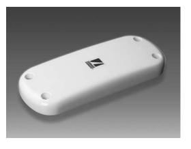
Dual-band active antenna operates at Globalstar<sup>™</sup> Frequencies, with continuous TX coverage from 1610 to 1626.5 MHz and RX band from 2483.5 to 2500 MHz. Receive side features a 29 dB gain amplifier with high-performance filtration and a built-in voltage regulator for DC bias operation of +3.3 to +28VDC.
