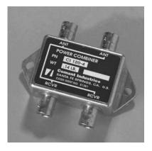
Two input—two output Power Combiner is standard for either antenna system. The Cl 120-4 provides for two separate cable runs to the avionics installation for NAV 1 and NAV 2 receivers. **P/N Cl 120-4**
