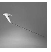
AM/FM receive antenna offers a unique low profile design using standard 4-hole mounting used on many VHF type antennas. Bent whip configuration is ideally suited for underbelly and helicopter installations. **P/N CI 222**
