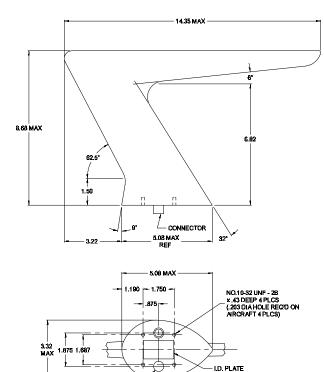
CONNECTOR CLEARANCE (.575 DIA HOLE REQD ON AIRCRAFT)
