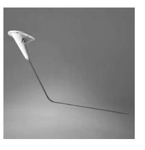
Designed to provide 2.5:1 VSWR or better over a bandwidth of 138 to 174 MHz. Features a high-strength die-cast 3-hole aluminum base. Radiating element is a bent-whip tapered stainless steel rod suitable for bottom mounting. The Cl 292-3 has been re-tested and upgraded to the new RTCA D0-160D environmental requirements. **P/N Cl 292-3**
