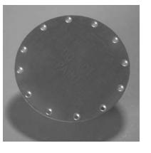
Flush mounted radar altimeter antenna encased in a 5.75" diameter aluminum die casting. Internal components are potted in place for mechanical integrity. Used in pairs, Cl 152s comply with ARINC 552 and exhibit very high isolation.
