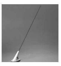
Wider band covers popular VHF and FM frequencies. Designed to provide 2.5:1 VSWR or better over a bandwidth of 138-174 MHz. Features a high-strength die-cast 3-hole aluminum base. Radiating element is a straight tapered stainless steel rod suitable for bottom mounting. Overall height only 14.5 inches with BNC connector as standard. The Cl 292-4 has been re-tested and upgraded to the new RTCA D0-160D environmental requirements **P/N Cl 292-4**
