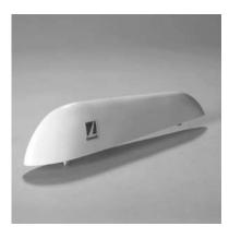
Designed for use with modern, high sensitivity marker beacon receivers. Small and lightweight, featuring 4-hole internal mounting for simple installation. Antenna assembly is enclosed in an injection molded radome which is impervious to the tough environments typical of the underside of an aircraft. Skydrol and rain erosion resistant. DC grounded to minimize accumulation of precipitation static.
