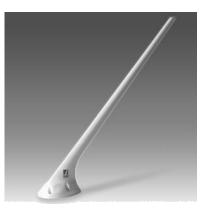
This sleek new design was developed for Cessna's 182 and 182T aircraft. Impressive with its low-drag and good looks, the Cl 248-5 has been credited with adding 2 to 3 Knots on certain aircraft. The first totally new look in VHF antennas in decades, the Cl 248-5 was tested to some of the most rigorous requirements outlined in RCTA D0-160D. Rated to 350 Knots for most high powered twins, the antenna is also certified for helicopter applications.
