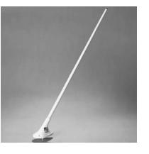
High strength antenna designed as an improved direct replacement for the standard Cessna 3-hole mounting configuration. The Cl 175 has been re-tested and upgraded to the new RTCA D0-160D environmental requirements and offers the 118 to 137 MHz frequency associated with D0-186A MOPS.
