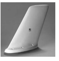
Designed for world-wide service where VHF communication is available over a wider band. Suitable for either top or bottom mounting. Solid Polyurethane construction for strength, reliability and durability. White Polyurethane finish is Skydrol and rain erosion resistant. The 108 Series has been re-tested and upgraded to the RTCA D0-160D environmental requirements. Optional leading edge protection available with the CI 108-1-L.
