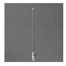
Stub antenna designed to withstand the harsh environments associated with the underside of an aircraft. Antenna radiator is mechanically captivated and is sealed against leakage. All exposed metal surfaces are nickel-plated for corrosion resistance and long service. Cl 271 mounts through single 0.600". BNC connector is standard. See Order Options for connector choices.
