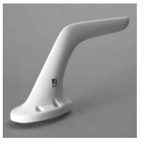
Optimum antenna for high-performance jet aircraft. Only 8.25" high, yet provides good performance without the added drag of a taller blade-type communication antenna. Skydrol and rain erosion resistant. The optional Cl 211-L offers leading edge protection as shown in outline drawing. The Cl 211 has been re-tested and upgraded to the new RTCA D0-160D environmental requirements and offers the 118 to 137 MHz frequency associated with D0-186A MOPS.
